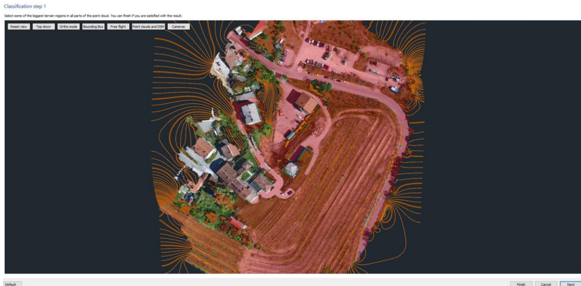
Figure 2: Points marked and filtered by increased values of Terrain Elevation and Terrain Slope
